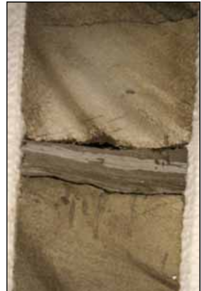
the Saline Aquifer Test Center project in Escatawpa, Mississippi. Note the shale stringer in the sandstone of the lower Tuscaloosa Formation.
